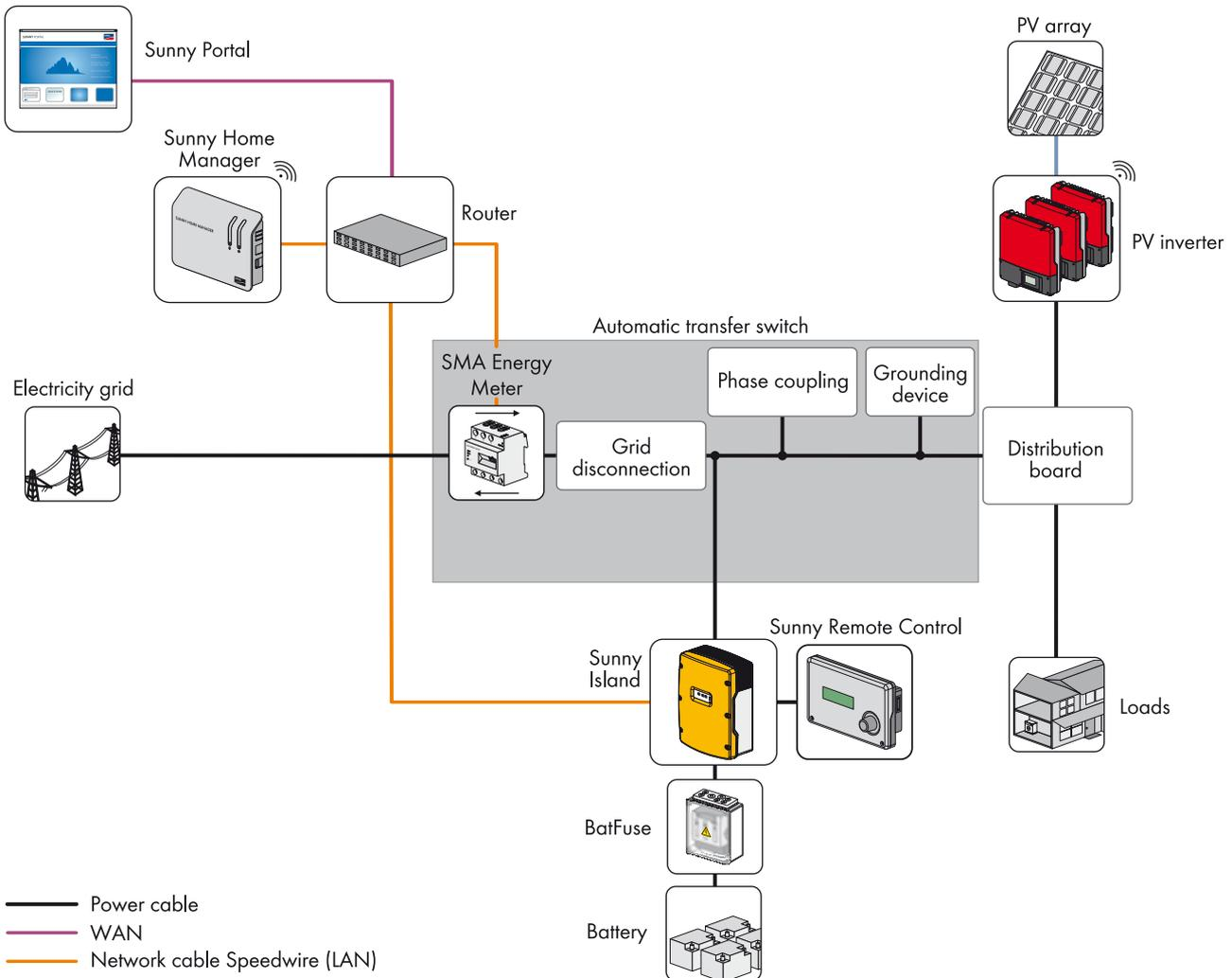
Figure 1: Overview of an SMA Flexible Storage System with battery-backup function
