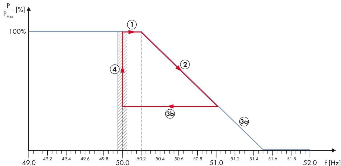
Figure 3: Suggestion for frequency-dependent active power limitation by the PV inverter (exemplary for Australia)
